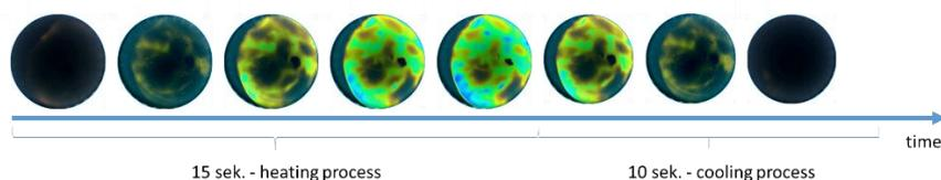
Figure 4. The process of heating after application and cooling down after putting away of the liquid crystal foil
