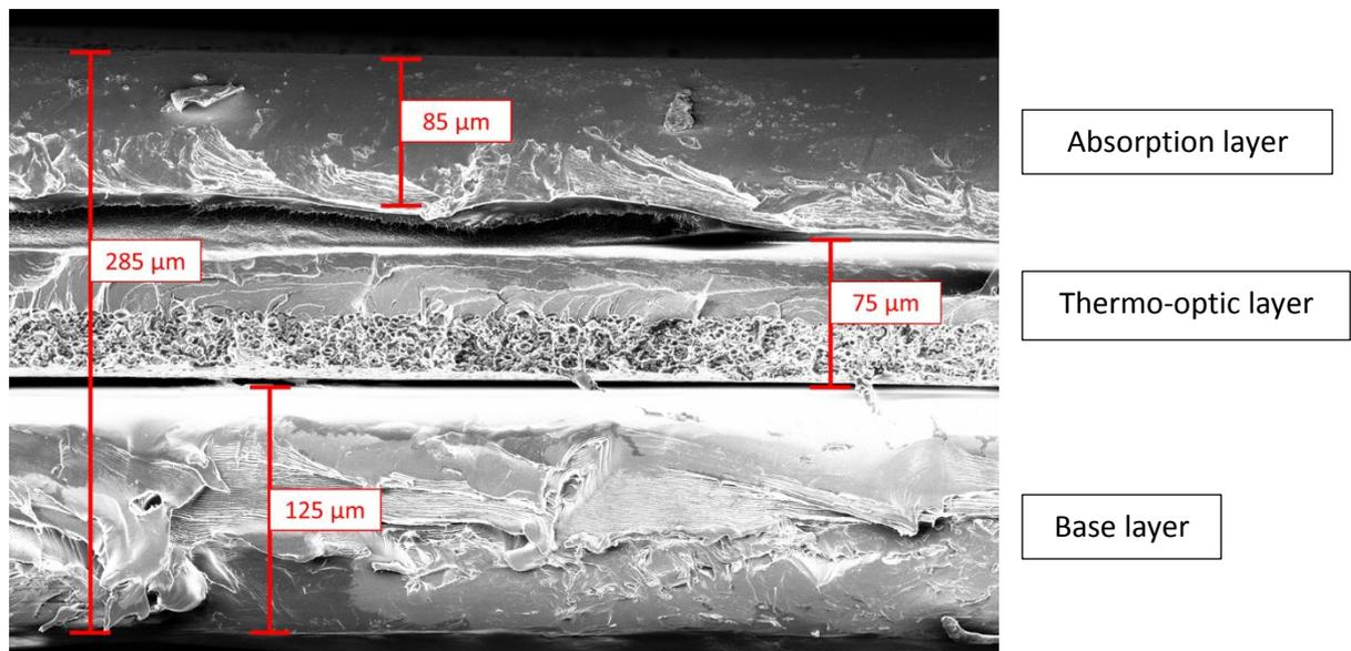
Fig. 2 Sectional view of the TLC matrix obtained with the electron microscope.
