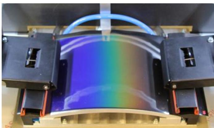
Fig.1 Thermographic film placed on a heating table
